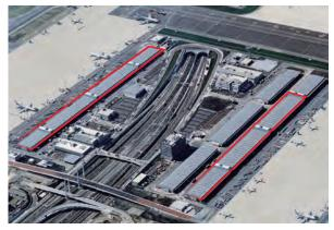
Red frame shows the area where the solar panels are installed.
